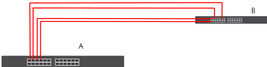
Figure 126 Trunking Example – Physical Connections
