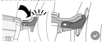
Try closing the door and check to make sure that it lines up with the control panel. If it does not, repeat the steps above: The door could become damaged if it does not work properly.
