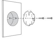
Route the cables through the square cable hole on the mounting bracket, and secure the mounting bracket to the junction box using screws. Then follow Step 4 and Step 5 of Option 2 to complete the installation.
