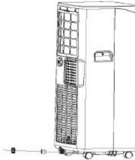
1. Continuous drainage (**Optional**) (only applicable to cooling and dehumidifying mode), as shown in figure:
