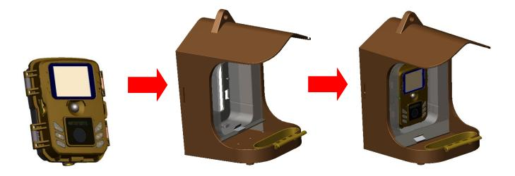
**Note:** ● Insert the power cable before inserting the camera to the camera holder through the power cord outlet. Pull the other end of the cable out of the outlet and then insert the camera from top to bottom into the camera holder of the container.
