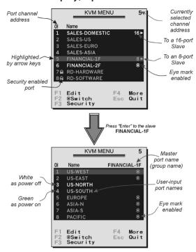
By hitting the left <CTRL> key twice within two seconds, you may see the 'Hotkey Menu' if it is enabled (an OSD option). Or, by hitting the left <CTRL> key three times within two seconds, you will see a 'KVM MENU' screen showing a list of the computers with corresponding channel addresses, names and status.
