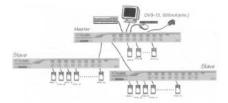
**NOTE:** A device (computer or KVM switch) at any 'PC x' port can be changed at any time after initial power-up. If you change any one of the **PC 1** to **PC 8** port connections from a computer to a Slave KVM switch or vice versa, or replace the devices of a port, the OSD will update this change the next time it is activated.
