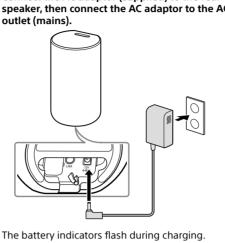
The battery indicators flash during charging. The battery indicators turn off after completion of charging.
