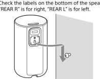
5 When mounting the rear speaker on the wall with the AC adaptor connected, fix the cable of the AC adaptor in the cable holder on the
