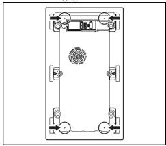
Fasten the fixing brackets (A) into the holes marked using the screws that were removed in order to correctly fix the hob to the structure.
