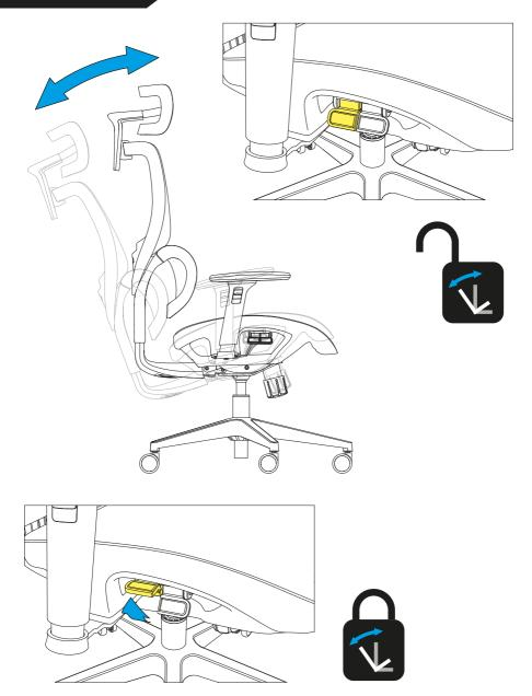
Once unlocked, slight pressure must first be applied to the backrest before the chair is released from the currently locked angle.
