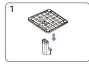
Put the stand base onto the stand neck as the direction shown in the figure.
