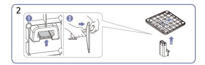
Push the hook in the direction shown in the figure and then pull the stand base to detach the stand as shown in the figure.
