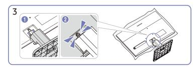
Place a soft cloth over the table to protect the product and place the product onto the cloth so that the front of the product is facing downwards. Push the assembled stand into the main body in the direction of the arrow as shown in the figure. Check that the stand neck is firmly connected.
