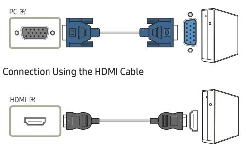
When connecting an HDMI cable, use the cable that came with the components of the product. If you use an HDMI cable other than provided by Samsung, the image quality may be degraded.
