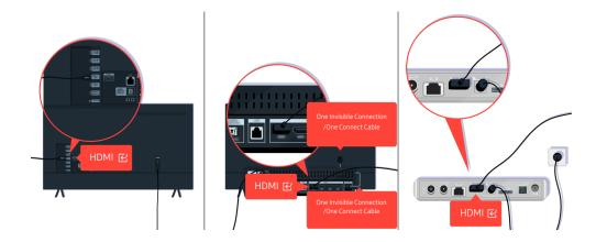
Check the connection of the HDMI cable to your TV or One Connect Box.
