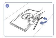
To disassemble the stand from the monitor, be sure to press the lower part of the monitor with one hand, and shake the stand from side to side with the other hand to make some gap between them.
