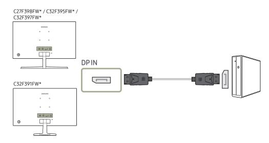
A DP cable shorter under 1.5m in length is recommended. Using a cable longer than 1.5m can affect the picture quality.
