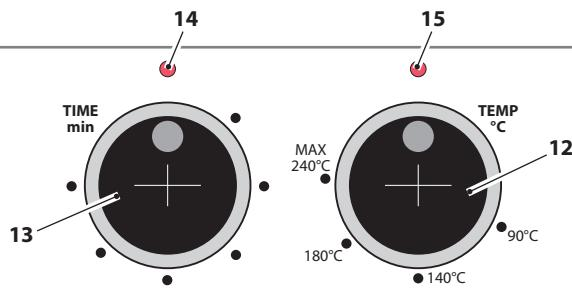
During cooking, the luminous LED (15) switches on and off, highlighting that the thermostat is maintaining the temperature set.
