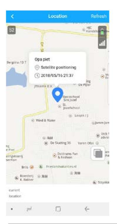
Users can set "Electronic Zone" under "Security"; after clicking "Position" can get updated position. The device will use any of LBS, Wifi, or GPS, according to signal density.
