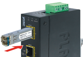
Figure 2-3: Plug-in the SFP Transceiver
