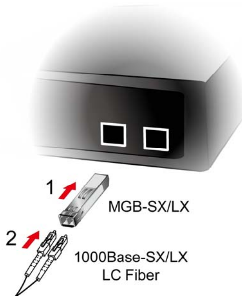
Figure 2-1-7 Plug in the SFP transceiver
