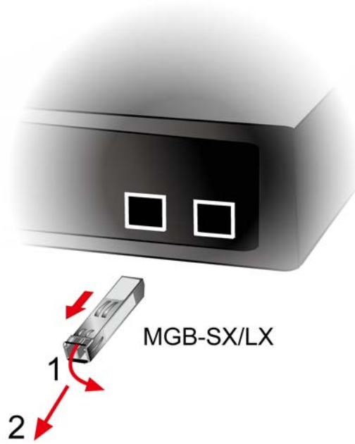
Figure 2-1-8 How to Pull Out the SFP Transceiver
