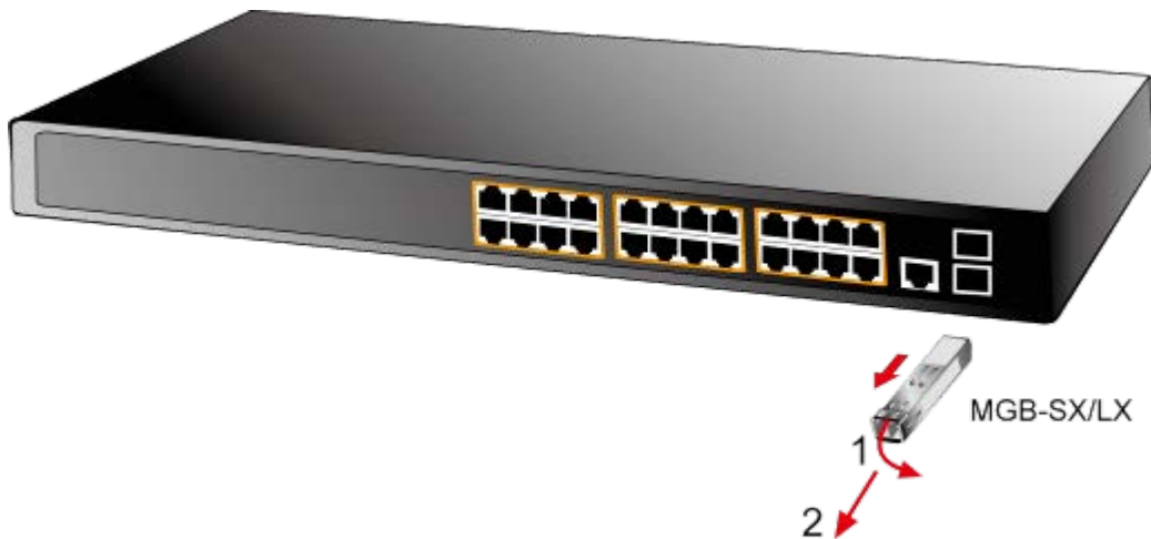
Figure 2-1-13: How to Pull Out the SFP Transceiver
