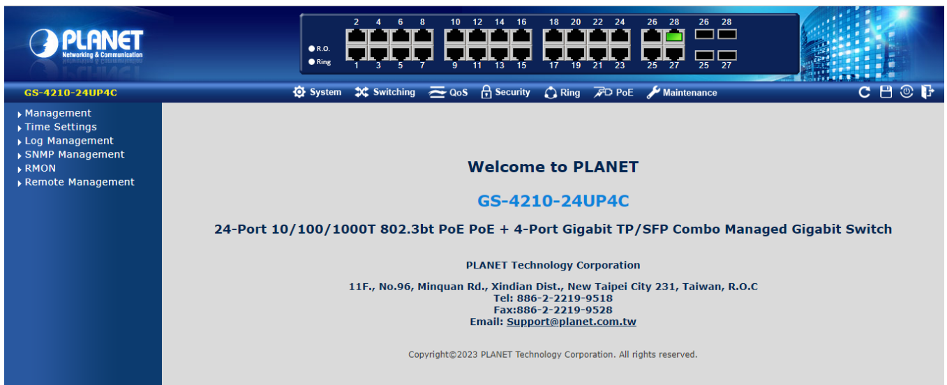
Figure 3-1-4 Web Main Screen of Managed Switch
