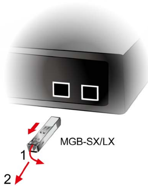
Figure 2-1-8 How to Pull Out the SFP Transceiver
