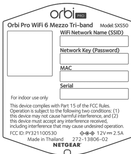
Figure 4. Orbi Pro WiFi 6 AX5400 SXS50 satellite label
