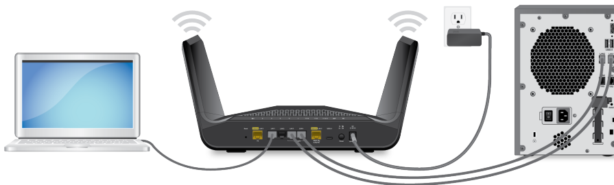
Figure 8. Ethernet port aggregation to a LAN device
