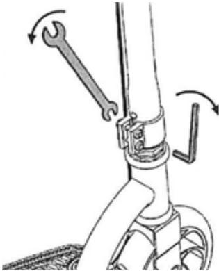
2. Tighten the bolts using the 5 mm hex wrench and the 10 mm wrench. Tighten the bolts evenly and securely.
