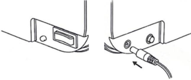
1. Make sure that the power switch, on the right side of the platform, is set to “0” before connecting the charger. Connect the charger to the charging port, which is located on the left side of the footrest. Set the switch on the right side of the footrest to “1”
