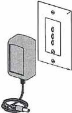
2. Plug the charger into a wall power outlet. The light on the charger housing should come on. A red LED light indicates that the battery is charging whereas a green LED light indicates that the battery is fully charged.
