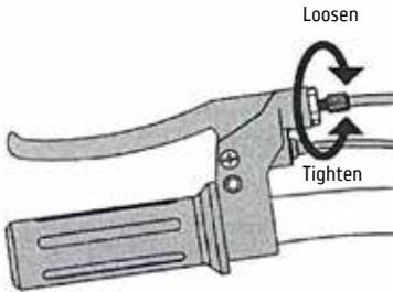
1. To adjust the brake cable, turn the adjuster barrel on the brake lever clockwise (to loosen) or counterclockwise (to tighten). Rotate the cylinder only a little at a time, until the desired adjustment is reached. If the brake still needs further adjustment, proceed to the next step.
