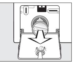
Remove the drain filter completely.
