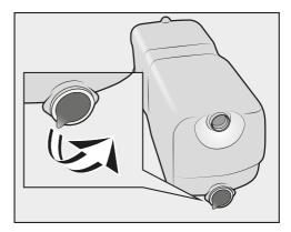
Remove the film from the detergent cartridges.
