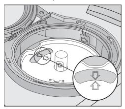
Put the holder back into place so that the arrows in the PowerDisk holder and in the viewing window point towards each other. The holder must lie flat. The AutoDos lid must close tightly so that the detergent powder does not get wet and clump together.
