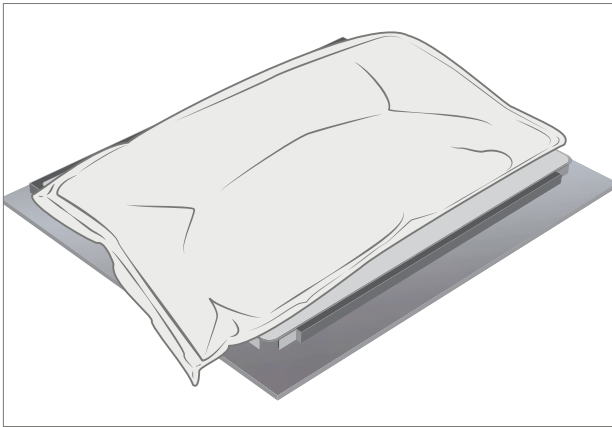
Place 9 kg steel shot bag onto device
