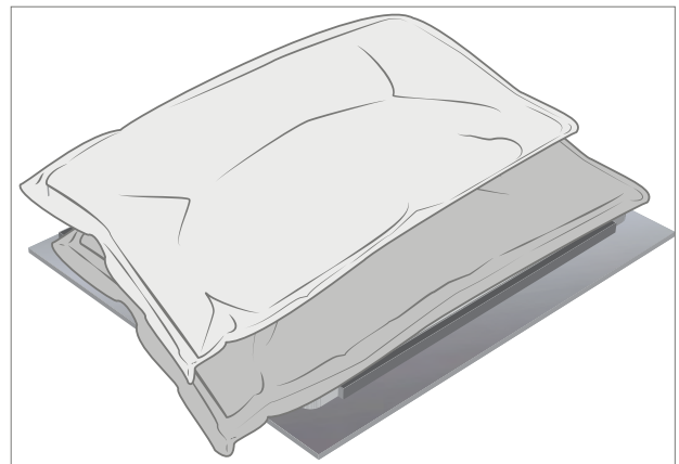
Shift second 9 kg steel shot bag to top edge of the device Bond for 3 minutes
