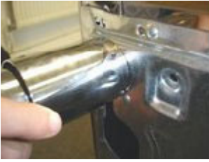
Figure5. Screw the leg up tight so the oven base is clamped between the washer and the top of the leg. Once all four legs have been fitted lift cooker onto the legs taking care to distribute the weight evenly onto all four legs at the same time. DO NOT tip the appliance onto its legs, always lift the appliance onto its legs. (This will require two people)
