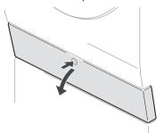
Remove the drain plug from the drain tube first and then drain the water. Then slowly unscrew the drain pump filter to drain the remaining water and then proceed to remove any debris or objects from the filter.
