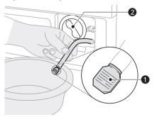
4 After cleaning the drain pump filter, carefully reinsert the filter and screw the drain cap back in clockwise carefully to avoid cross threading and leakage. Reinsert the plug back into the drain tube and place the tube into its holder. **5** Close the lower cover.
