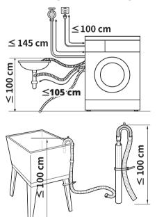
If the drain hose is too long, do not force it back into the appliance. This will cause abnormal noise.  When installing the drain hose to a sink, secure it tightly with string.
