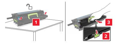
Unpack the new developer unit, and then remove the packing material.
