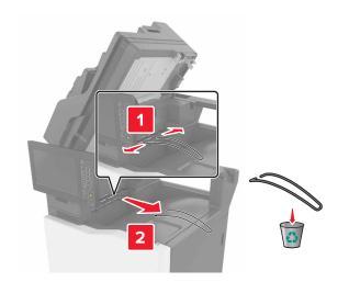
**4** Remove the paper transport and staple finisher connector covers.
