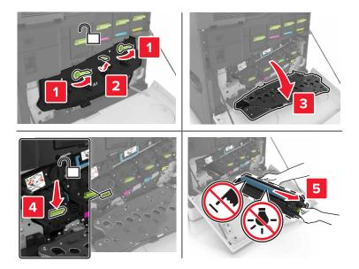
**5** Remove the photoconductor unit.
