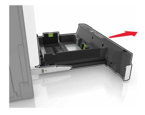
Remove the separator bracket.
