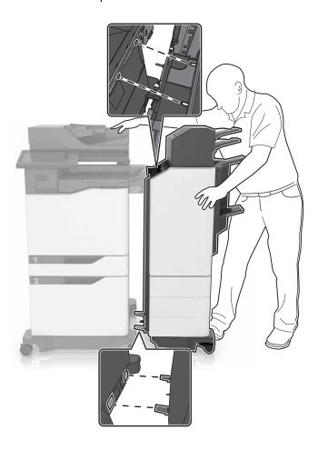
**14** Push the finisher to the printer, and then apply pressure with your foot at the bottom of the finisher until it *clicks* into place.
