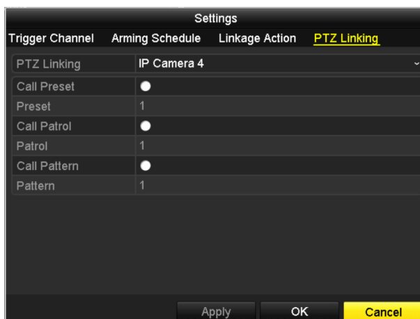
Figure 8. 7 Set PTZ Linking of Alarm Input
