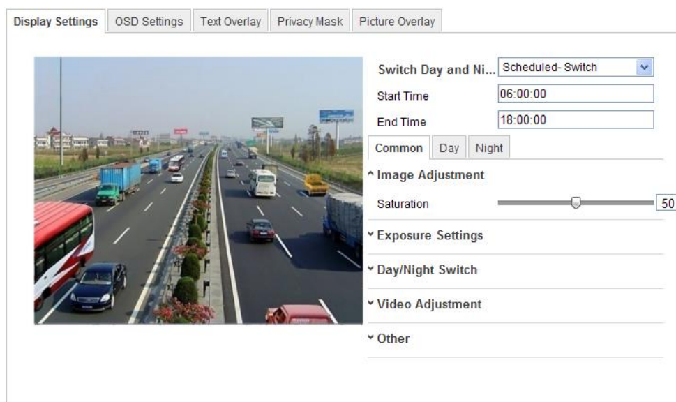
Figure 6-35 Day/Night Scheduled-Switch Configuration Interface
