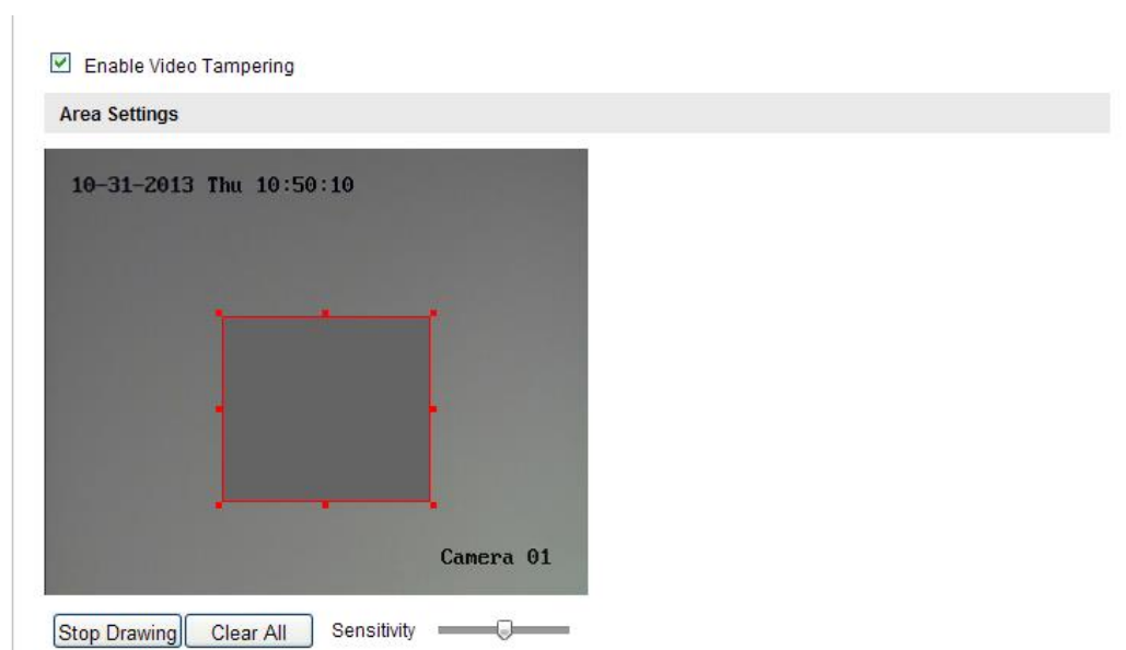
Figure 6-49 Video Tampering Alarm
