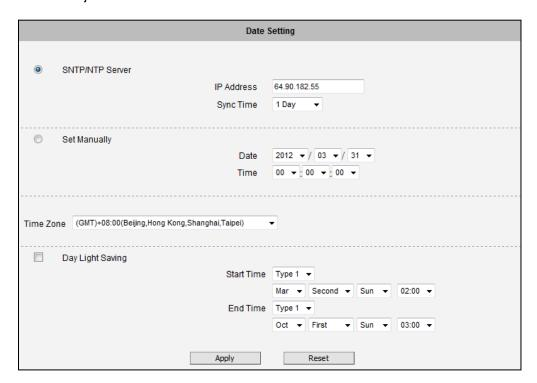
When choosing **SNTP/NTP Server** for automatic date and time updating, you can key in the IP address of the NTP server and the time interval for automatic time synchronization. If you want to key in the domain name of NTP server instead, please make sure the DNS server IP address has been set under IP Settings; otherwise the camera will not be able to resolve the domain name of the NTP server.
