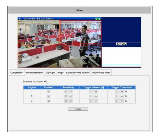
Click on "Setup" to adjust the motion detection regions or its parameters. **Microsoft Internet Explorer** browser is required to configure the motion detection regions.
