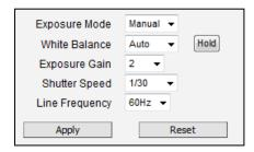
In manual exposure mode, the user can directly adjust the signal gain and shutter speed manually. The White Balance and Line Frequency controls have already been explained in the previous chapter.
