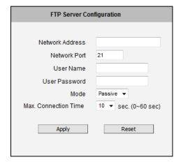
To setup FTP servers, make sure to enter the network address of FTP server, the Network (FTP) port, the User Name and Password of FTP account, Connection mode (Passive or Active) and Connection time before timeout.
