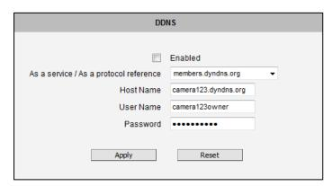
To activate DDNS, please check the "Enabled". Select the service reference, input the Host Name (the domain name given to the camera by DDNS service, User Name and Password of the DDNS server account.
