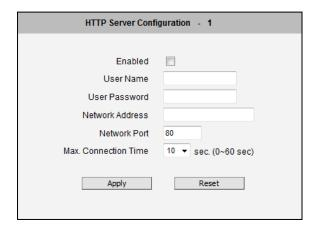
To setup HTTP servers, make sure to enable the HTTP server, enter the user name, the user password, Network (HTTP Server) address, Network (HTTP Server) port number and Max connection time before timeout (in seconds).
