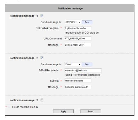
To setup Notification Messages, make sure to enable the message and then determine what type of message to send (HTTP CGI or email).
