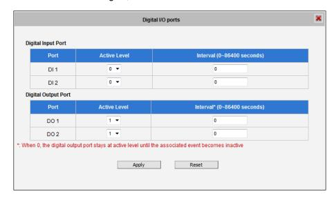
The Digital I/O Ports page displays the number of available DI and DO ports on the camera, which varies depending on camera model.
