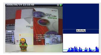
The blue graph on the right side of the image shows how many percent of pixels within the motion detection
