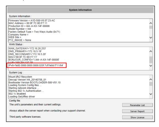
To access the camera with the IPv6 address, type the IPv6 address enclosed in square brackets on the web browser address bar. For example:
