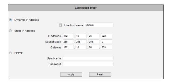
**Host Name** is used to identify the camera by a DHCP server. In some networks with very strict security policy, it is required that all the network devices should have their host name, and when the devices attempt to access the network by requesting an IP address from a DHCP server, the DHCP server would check if the host name is among the allowed devices. On this page, it is possible to edit the Host Name and enable or disable the use of host name.
