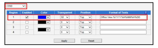
In the example above, one region of text was enabled with blue color and 50% transparency, located at left lower corner and containing the text of "Office View" together with current date. The date would be automatically changing every day, according to camera's date and time settings. The result of the example configuration would look like this (Live View page, 1:1 scale):
