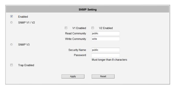
The SNMP agent supports versions V1, V2 and V3. SNMP V1 is the initial implementation of SNMP. SNMP V2 is proposed to enhance the performance of management, such as the communication of server and devices, the confirmation of information delivery and receipt. Primary additions in SNMP V3 concern security and remote configuration enhancements.
