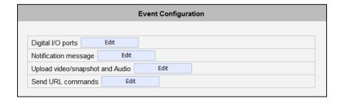
NOTE: Digital I/O ports appear only for the camera models that support this function.
