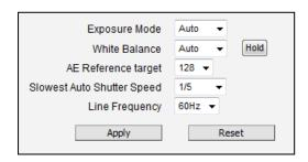
In Auto Exposure Mode, you control the image brightness by configuring the AE Reference Target and Slowest Auto Shutter.
