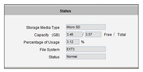
In case of IP cameras with installed memory cards, the Storage Media Type will show "Micro SD".
