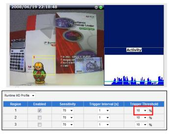
The blue graph on the right side of the image shows how many percent of pixels within the motion detection
