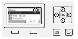
When [OK] is displayed, selecting the [OK] key will confirm the selection. Selecting the [Back] key will return to the previous level in the menu.
