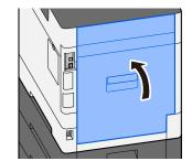
**3** Open the Rear Cover 2 and remove the jammed paper.
