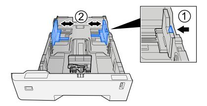
2 Adjust the paper length guide to the paper size required. Press the paper length adjusting tab and slide the guides to the paper size required.
