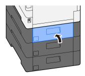
**3** Open the Rear Cover 3 and remove the jammed paper.
