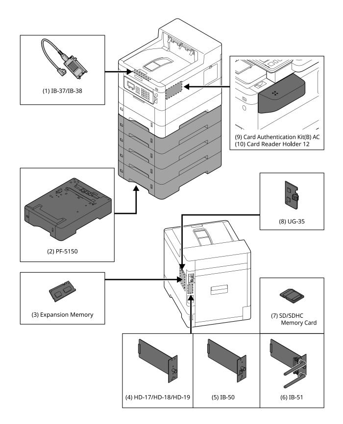
1 IB-37/IB-38 <Wireless network interface (USB: 5GHz/2.4GHz)>
