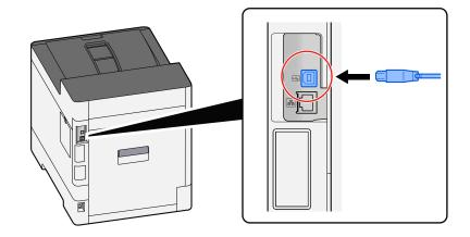
2 Connect the other end of the cable to the PC.
