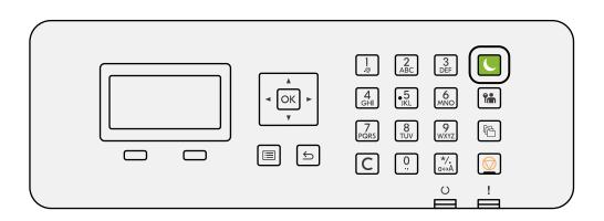
If print data is received during Sleep, the machine automatically wakes up and starts printing.
