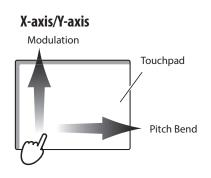
Press the Pitch/Mod button to switch the Touchpad to the Pitch/Mod mode.
