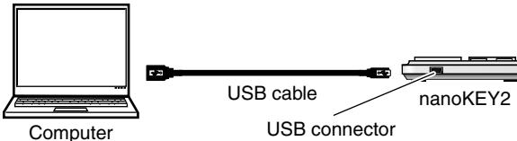
1. Use a USB cable to connect the nanoKEY2 to a USB port on your computer. The power to the nanoKEY2 will turn on and the power LED will light up.
