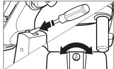
Lift motor head. Turn screw slightly counterclockwise (left) to raise flat beater or clockwise (right) to lower flat beater. Make adjustment with flat beater, so it just clears surface of bowl. If you over adjust the screw, the bowl lock lever may not lock into place.
