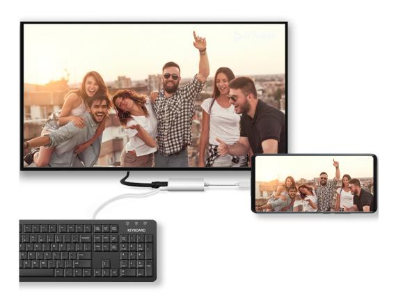
**3** On the external display, set the corresponding HDMI, DP, or MiniDP input as the signal source.
