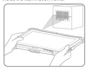
4. Release the button when the computer beeps. The barcode information is entered into the application in use.
