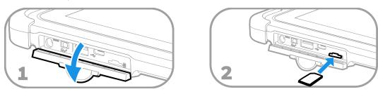
**Note:** Always power off the tablet before attempting to install or remove a card.
