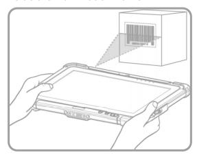
7. Release the Scan button when the computer beeps. Barcode information appears on the screen.
