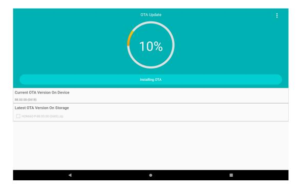
9. Once the installation is complete (100%), select **OK** when prompted to **Reboot** the computer. The computer reboots and finishes the update.
