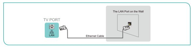
If you have a Dynamic Network, you should use an ADSL modem or router that supports Dynamic Host Configuration Protocol (DHCP). Modems and routers that support DHCP automatically provide the IP address, subnet mask, gateway, and DNS, so you don't have to enter them manually. Most home networks are Dynamic Networks.
