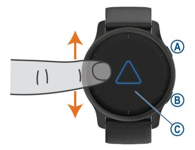
Action button: Hold to turn on the device.
