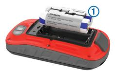
3 Insert the battery pack, observing polarity.
