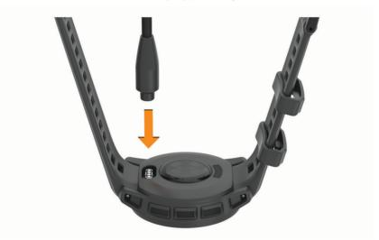
2 Plug the large end of the USB cable into a USB charging port. The watch displays the current battery charge level.
