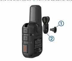
2 Secure the spine mount adapter ① over the back of the device using the long screw ② included with the device.
