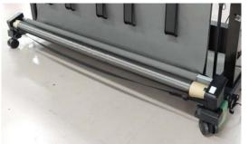
Remove the optional auto take-up reel unit or SpectroProofer mounter if they are installed.
