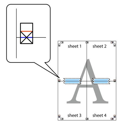
8. Cut the taped sheets in two along the horizontal red line through the alignment markers (this time, the line above the cross marks).
