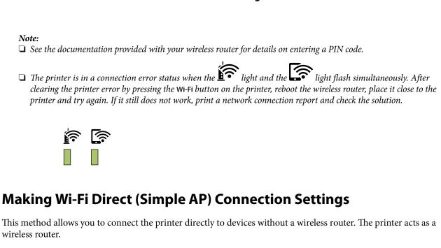
1. While holding down the Wi-Fi button, press the button until the light and the light flash
