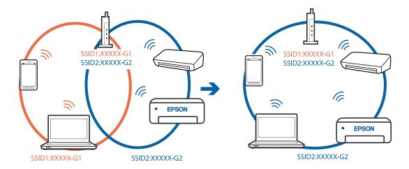
□ A wireless router that is compliant with both IEEE802.11a and IEEE802.11g has SSIDs of 2.4 GHz and 5 GHz. If you connect the computer or smart device to a 5 GHz SSID, you cannot connect to the printer because the printer only supports communication over 2.4 GHz. Connect the computer or smart device to the same SSID as the printer.
