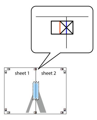
3. Cut the taped sheets in two along the vertical red line through the alignment markers (this time, the line to the left of the cross marks).
