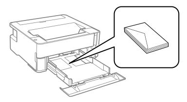
☐ Fan and align the edges of the envelopes before loading. When the stacked envelopes are puffed up with air, press them down to flatten them before loading.
