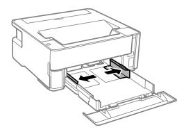
With the printable side facing down, load paper until it touches the back of the paper cassette.
