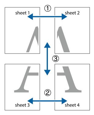
1. Prepare Sheet 1 and Sheet 2. Cut off the margins of Sheet 1 along the vertical blue line through the center of the top and bottom cross marks.
