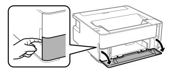
2. Check that the printer is not operating, and then slide out the paper cassette.
