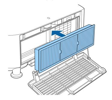
**5** Replace the air filter cover as shown and tighten the screws.
