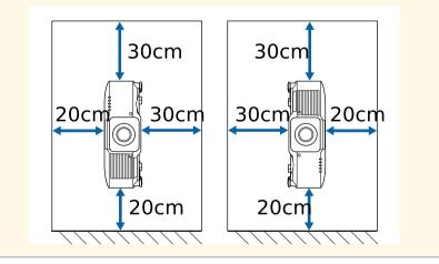
Installation space (When installing multiple projectors side by side)
