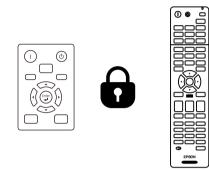
Even if you can lock the buttons on the control panel, you can still use the remote control as usual.
