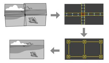
You can easily and quickly create a single seamless image from multiple projectors when projecting on a flat screen.
