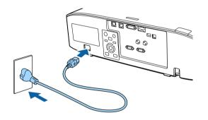
The projector's power indicator turns blue. This indicates that the projector is receiving power, but is not yet turned on (it is in standby mode).
