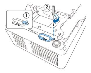
2 Loop the safety wire through the hole in the ceiling mount, and then attach both ends to the carabiner.
