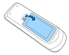
**2** Remove the old batteries, if necessary.
