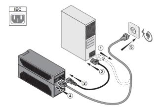
Connect the UPS to the AC-power source with cable through a wall outlet equipped with an earth connector, using your equipment cord.
